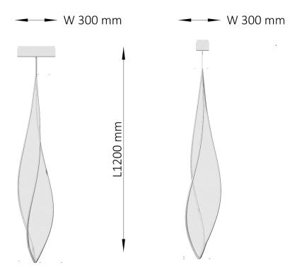
golden coloured polyester with metal fabric stretched around bended rods containing the led tape of 330cm 30Watt
