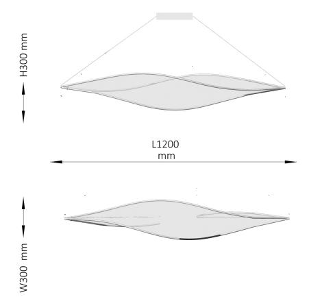
golden coloured polyester with metal fabric stretched around bended rods containing the led tape of 330cm 30Watt
