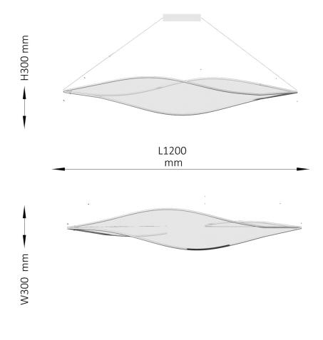
white polyester with metal fabric stretched around bended rods containing the led tape of 330 cm 30Watt
