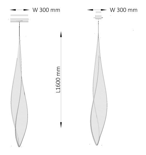
golden coloured polyester with metal fabric stretched around bended rods containing the led tape of 500 cm 50 Watt
