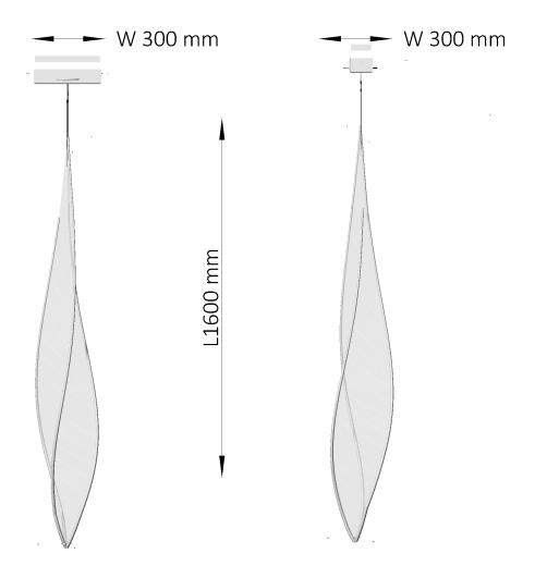
white polyester with metal fabric stretched around bended rods containing the led tape of 500 cm 50 Watt
