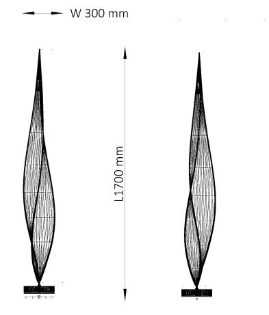
white polyester with metal fabric stretched around bended rods containing the led tape of 500 cm 50 Watt
