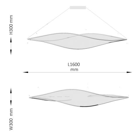
golden coloured polyester with metal fabric stretched around bended rods containing the led tape of 500 cm 50 Watt
