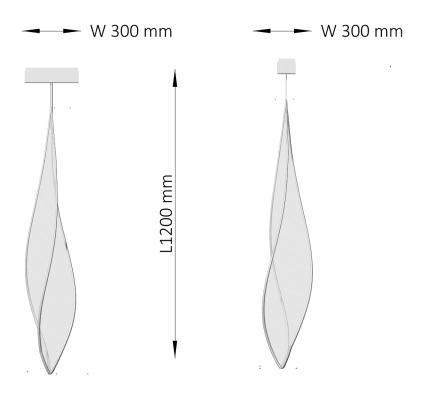
white polyester with metal fabric stretched around bended rods containing the led tape of 330 cm 30Watt
