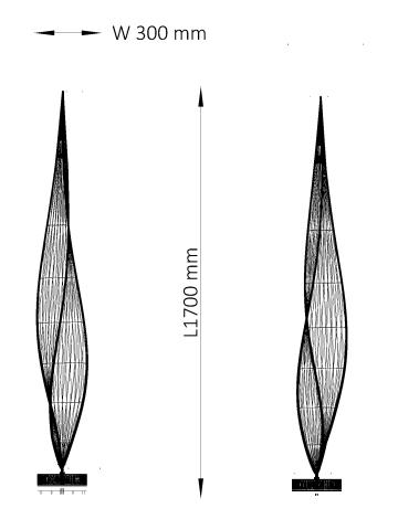
golden coloured polyester with metal fabric stretched around bended rods containing the led tape of 500 cm 50 Watt
