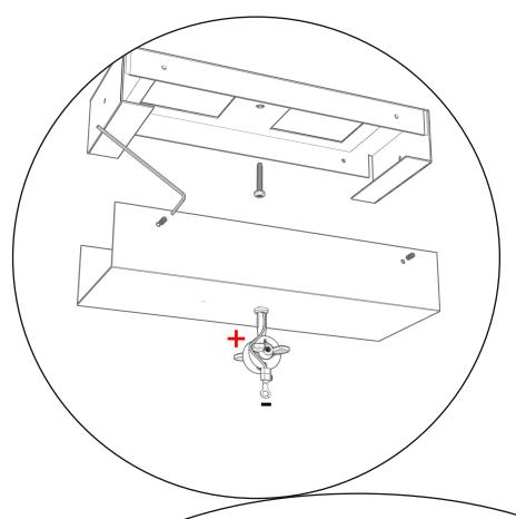
Mount the top part of the canopy on the ceiling. Connect the blue and brown cables of the
